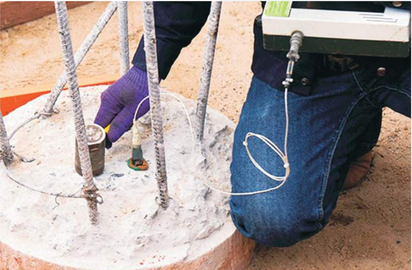
PILE INTIGRITY TEST for 3000 Numbers of Foundation pile ( 600 mm & 700 mm diameter ), Depth - 12 mtr., at Sunteck City, Phase I and Phase II, Naigaon, **SUNTECK REALTY LTD.**
