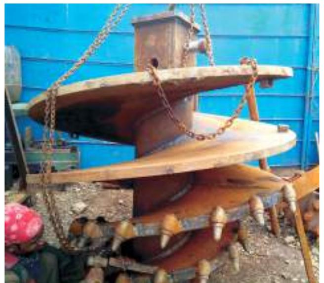
Making of M.S. Liner & Rock Augar up to 1500 mm Piles at **WORKSHOP**
