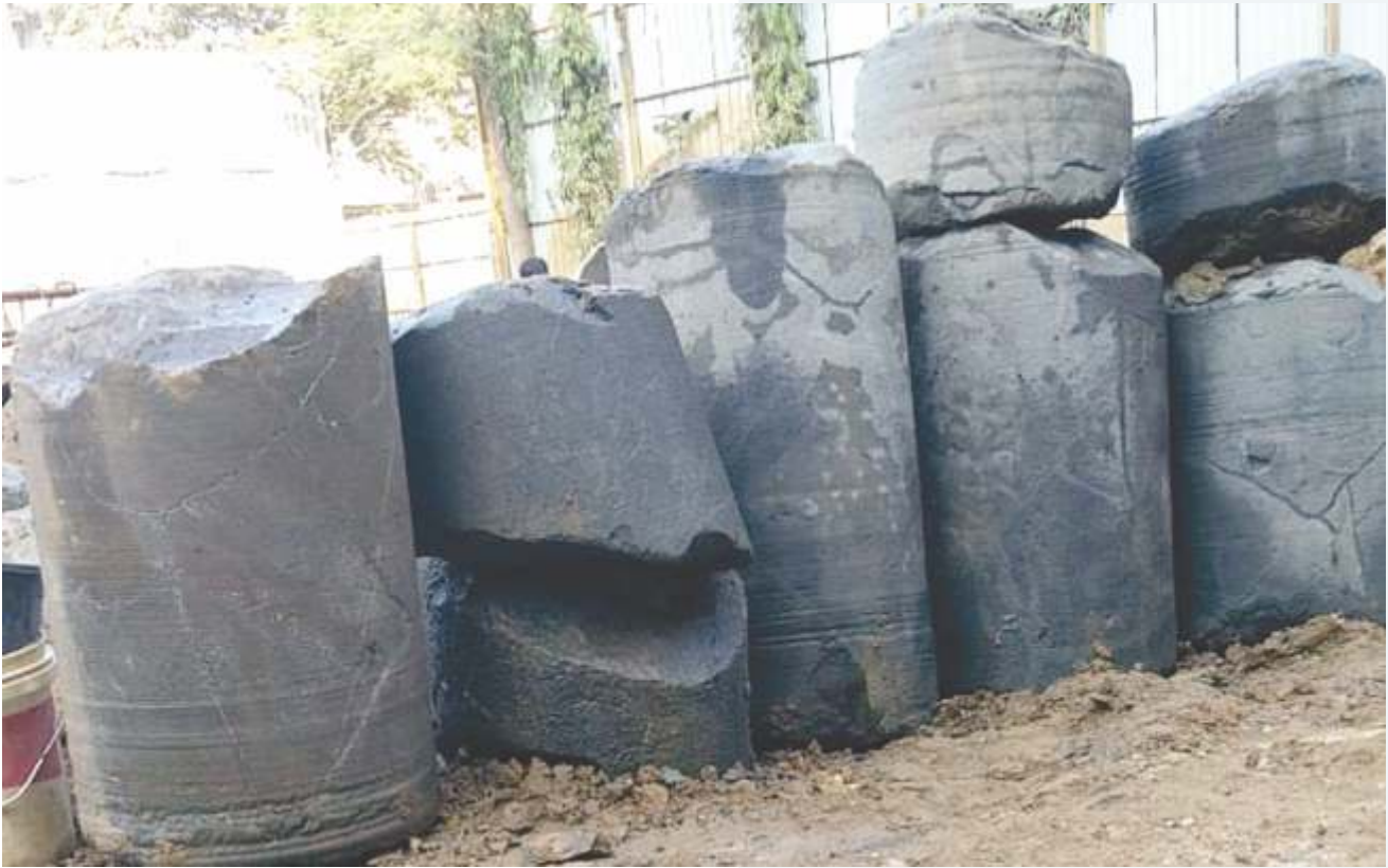
BASALT CUTTING WITH CORE BARREL
