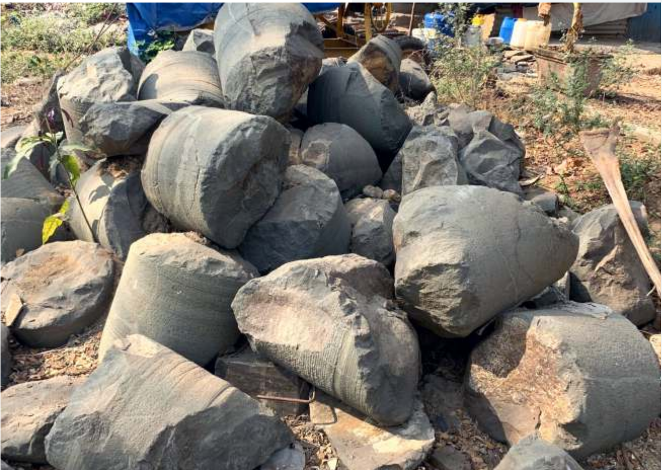
BASALT CUTTING WITH CORE BARREL
